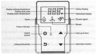
Each time you press the " ^ " key, the temperature will drop by 1 °C and the temperature drops by 1 °C every 0.25 seconds while you keep pressing this key continuously.
